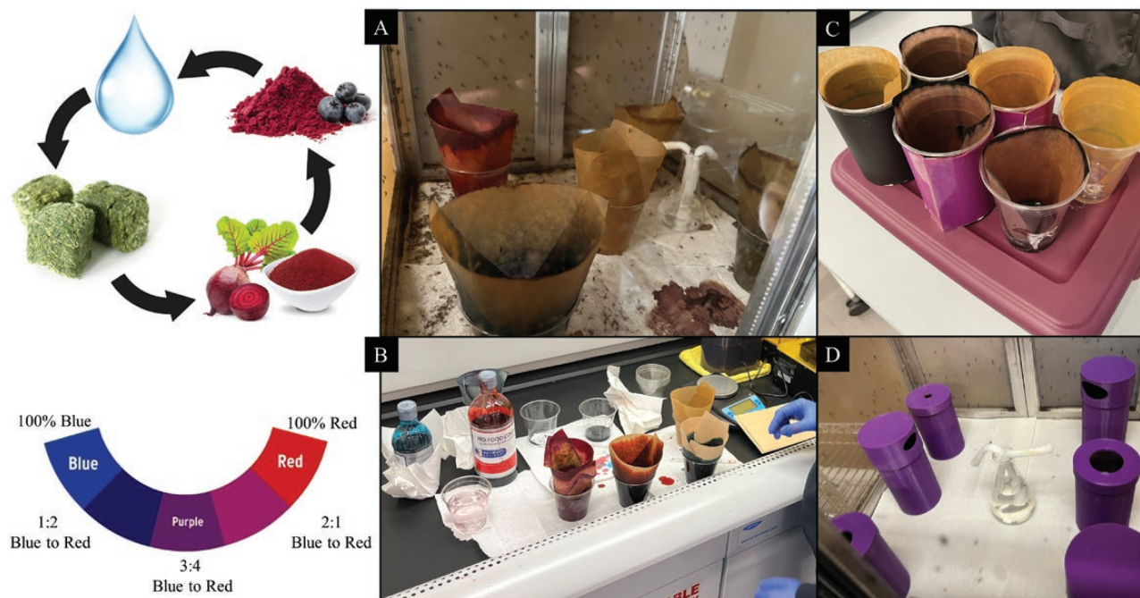
Fig. 1. A) Infusion additives choice assessments; B) Red-to-blue spectrum tests; C) Pairings for purple versus black cups and purple versus clear water; D) 3D-printed ovicup prototype with top or side entry for small, medium, and large holes.
