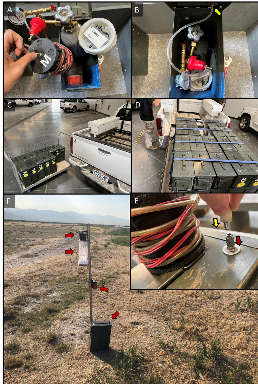
Fig 4. A) Ammo can transport a filled CO 2 cylinder with regulator, trap fan with airstone, trap net with label, and battery; B) ammo can packed together; C) transport and load; D) squared design fits into racks on a truck bed-slide system; E) trap-to-can CO 2 connection; F) Fully deployed trap with 6v battery and trap secured to pole and linked with ammo can.
