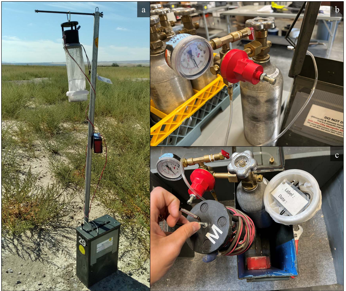
Fig. 2. (a) A field-deployed Salt Lake City (SLC) mosquito trap with contained transport and housing for gas cylinders. This unit is functionally equivalent to miniature CDC-style traps. (b) Regulator attachment to gas cylinders are fed through transport housing. (c) Cargo of battery, trap, trap net, cylinder, and attached regulator are packaged into the housing for transport.
