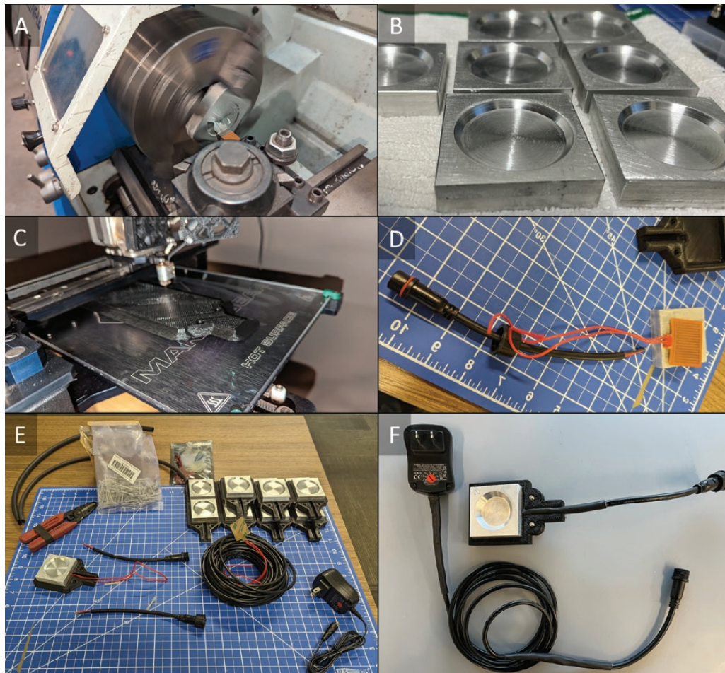
Fig. 1. A) 5 × 5 × 1.3 cm solid aluminum square routed for a 3.8-cm-diameter well; B) aluminum wells with 0.16–0.32 cm depths, depending on needs; C) 3D-printed housing for mounting heater, wiring, and aluminum can be substituted for any cut housing with metal or plastic; D) 6-volt film heater with adhesive pad to adjoin the aluminum and quick connect wire harness to bridge to adapter; E) partial assembly of all components, showing option to extend wire length based on needs by braiding in additional equivalent gauge wire; F) final assembly.
