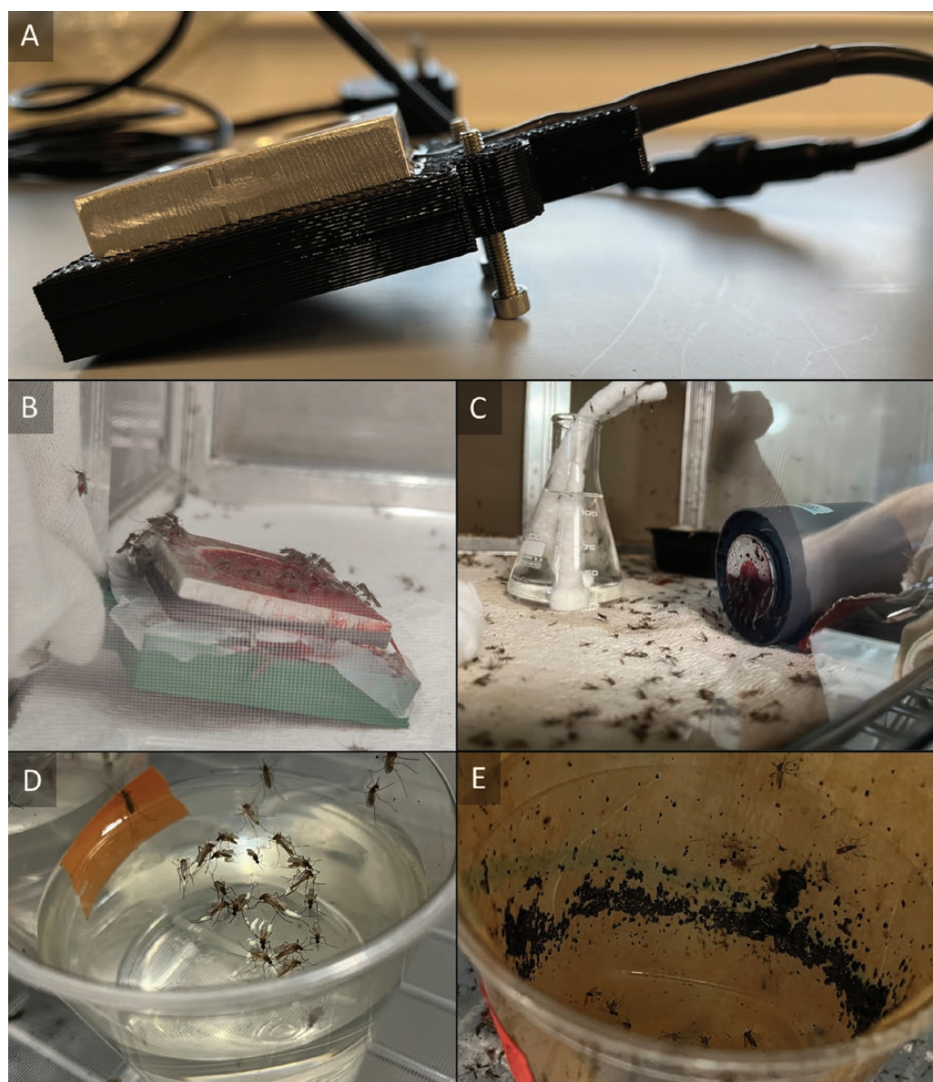
Fig. 2. (A) Angle screws in the SLAMto allow height adjustment; B) MAD blood-feeder presented at an angle; C) Hemotek blood-feeder presented vertically; D) Culex pipiens egg raft assessment; E) Aedes aegypti egg paper assessment.
